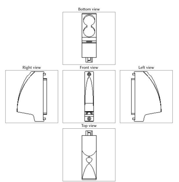
Modicon M340 automation platform - Removable connection blocks and preformed corsets for I/O modules - Type: Cordons, connection: 1 40-way connector, number of sheaths: 2 x 20 wire (32 channels), length: 3 m Product datasheet
