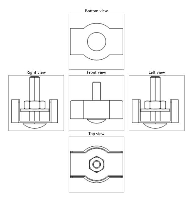
Emergency stop rope pull switches Preventa XY2C, cable grip
